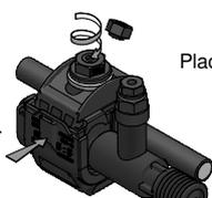
Place the connector on the main conductor and tighten with a 13mm hexagonal wrench until shear-head breaks. 15 Nm.
