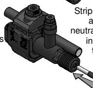
Strip the tap conductor over the advised length, brush it with neutral grease, then insert it fully in the bore. **Do not unscrew the screw on the tap side, this one is correctly positioned in factory.**
