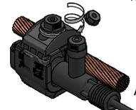
Tighten the tap contact screw with a 13 mm hexagonal wrench until shear-head breaks. 15 Nm.
