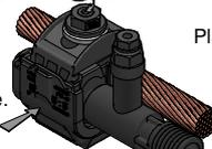
Place the connector on the main conductor and tighten with a 13mm hexagonal wrench until shear-head breaks. 15 Nm.
